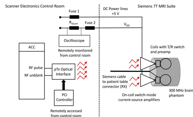
**Figure 3:** Hardware setup in scanner for human brain imaging.
