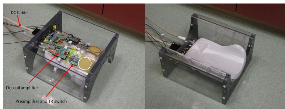
**Figure 2:** Preliminary 2-channel on-coil TX/RX head array.
