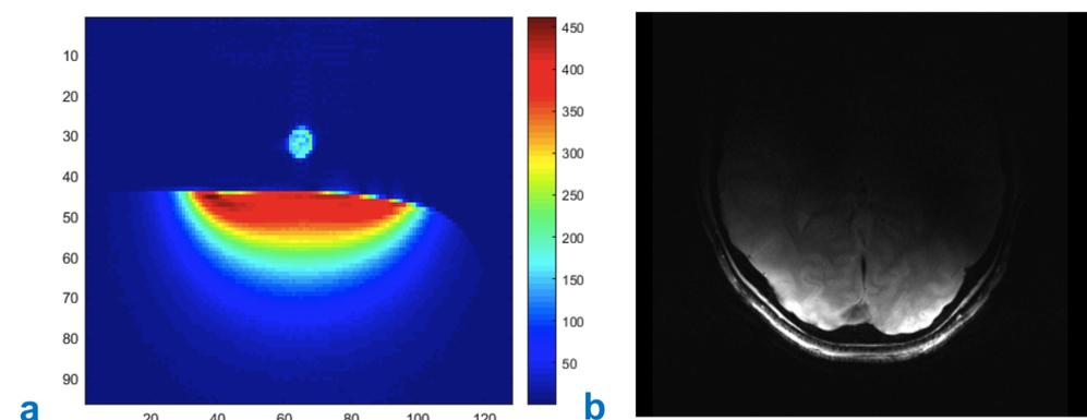
**Figure 4:** Test of new TX-RX hardware in the scanner. **a)** SNR map of oil phantom acquired with a single on-coil transceiver. **b)** Image of the occipital brain area from the combined signal of two RX channels.
