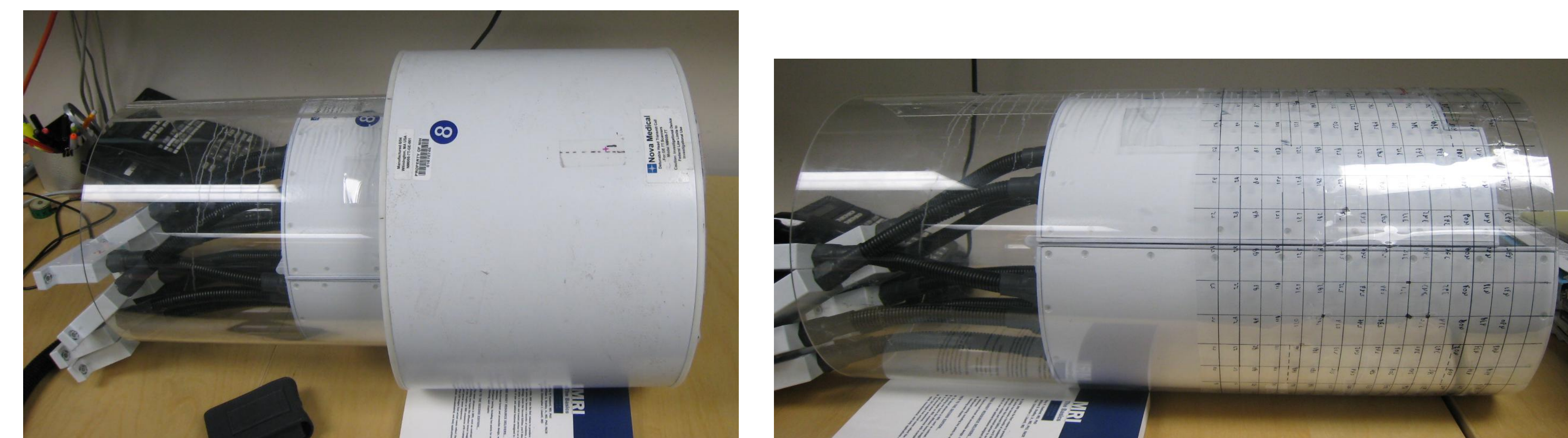
Figure 1: Pictures of the proposed passive shimming construct currently being constructed. The shim elements will be mounted on an acrylic cylinder inserted between the transmit and receive-array coils (left). A 16x32 grid of particles is used (right).
